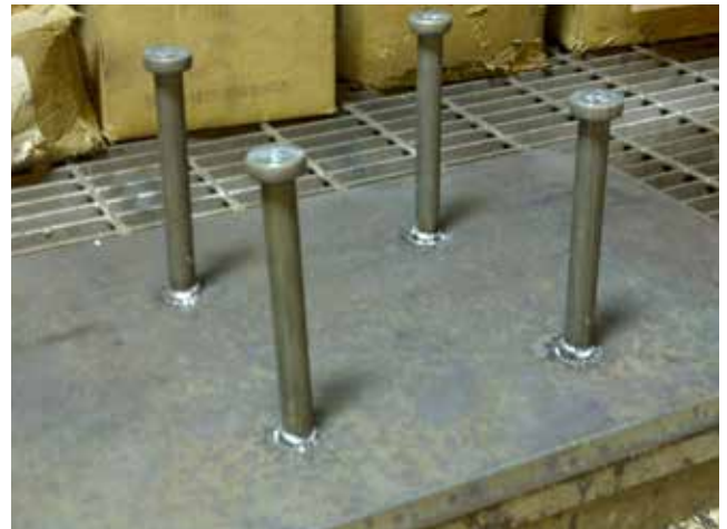
▲ Shear studs on embedded plates.
