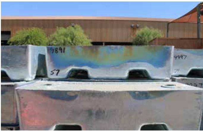
► Zinc arrives at the facility in approximately 2,400-lb pieces and is added to the kettles regularly as the levels get low; the operators keep the level 2 in. to 3 in. below the lip of the kettle to prevent spillage when elements are dipped. This facility has three kettles in two different buildings, as well as a decommissioned kettle. The two longest kettles—43.5 ft long and 36 ft long—are both 6 ft wide and 9 ft deep, while the third kettle is 23 ft long, 3 ft wide and 6.5 ft deep.
