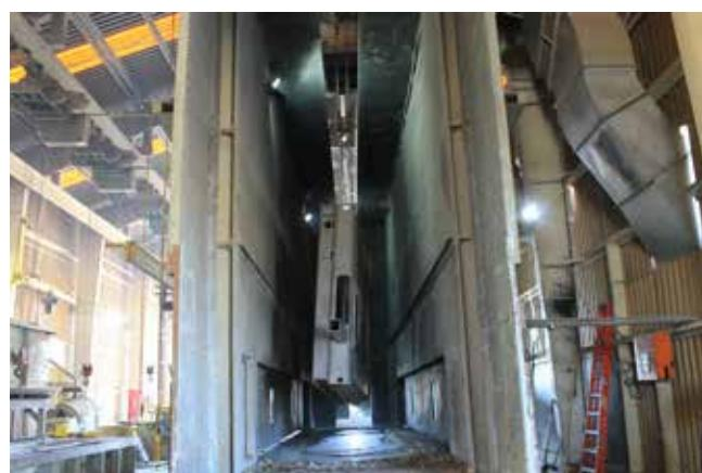
▲ The galvanizing process was discovered in the 1700s and the basics haven't changed much since. The mixture that the steel is dipped in is 99% pure zinc, along with a small amount of aluminum (which gives it a shine) and other proprietary chemicals.
