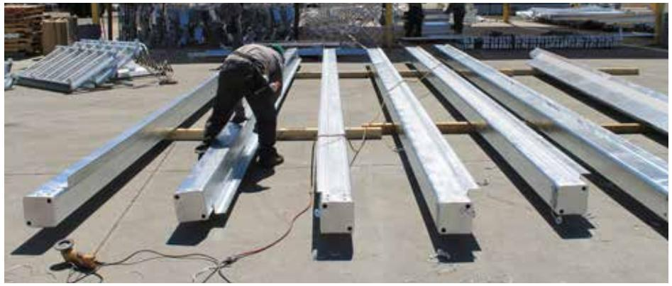
▲ Once the steel is galvanized, quality control is essentially built in, as defects or voids in the coating are visible to the naked eye. Deburring is performed outside as necessary.
