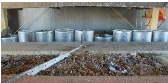
▲ All zinc used at the plant is 100% recyclable. AZZ removes a slag material called "dross" from the kettles about every two weeks. Dross is created from small particles of iron coming off the steel being dipped; the iron particles are encapsulated by zinc, and because they're heavier than zinc, fall to the bottom of the kettle. The dross is compressed into blocks and sold to a company that separates the zinc from the iron, then sells the zinc back to the galvanizer.
