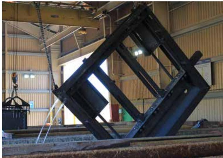
▶ From the pickling tank, the batch goes into another water bath to rinse off the acid. The next and final bath before the actual zinc dip is a low-pH zinc ammonium chloride mixture, which acts as a fluxing agent. It also contains a chlorine salt that encapsulates the metal and prevents it from oxidizing again.
