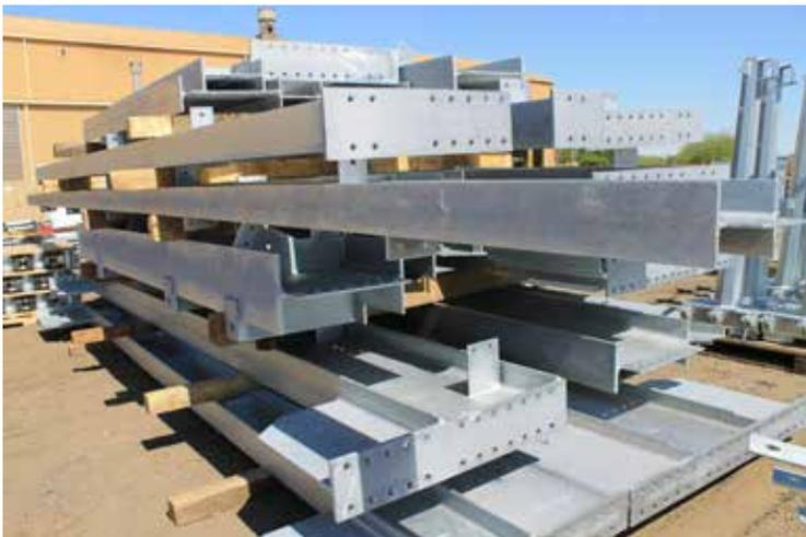
◀ The turnaround time for a galvanizing job, from the time it arrives from the fabricator to when it is ready to be shipped to a project site or service center, is typically five days.
