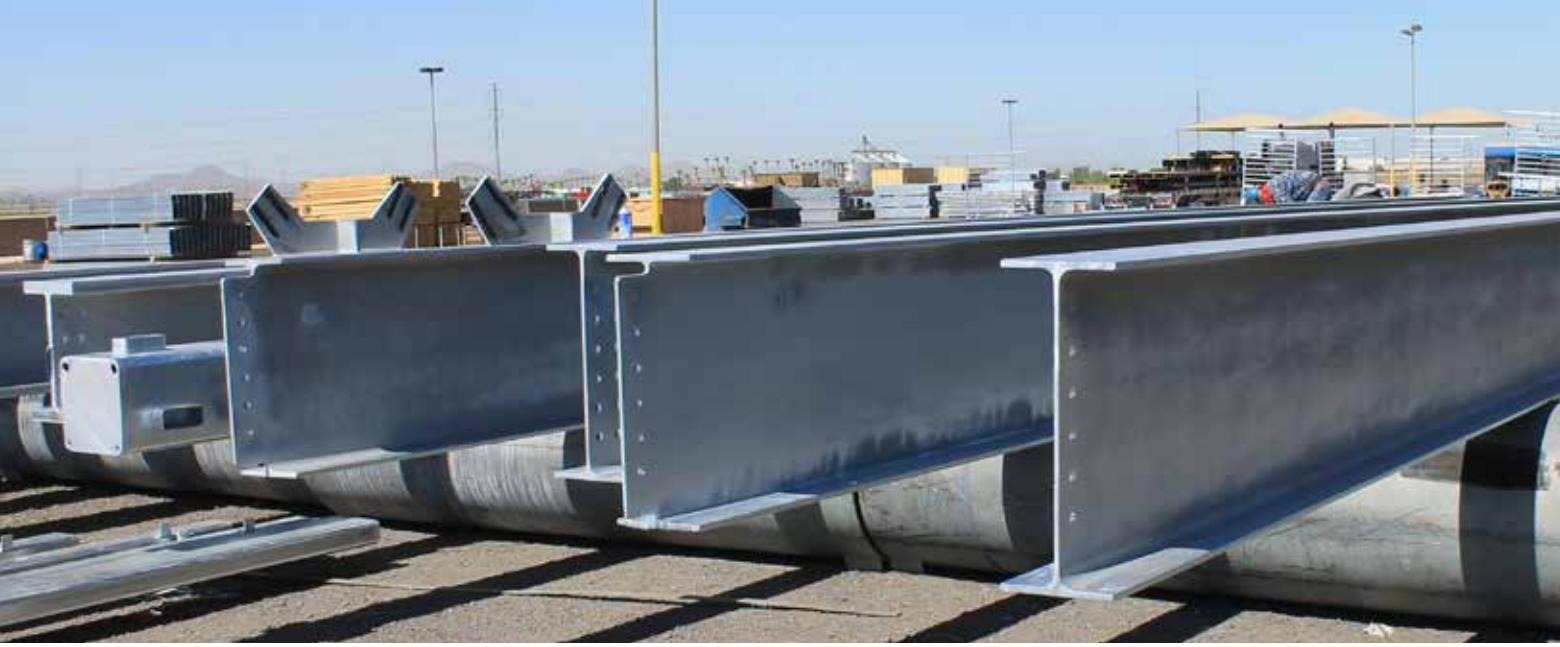
**HOT-DIP GALVANIZED STEEL**, known for its silver-gray hue, sports a protective zinc coating that prevents oxidization. Zinc and iron react to one another through a diffusion process, creating a four-layer zinc iron alloy. This layer of protection is particularly suitable for steel that must withstand harsh, outdoor environments where it is exposed to the elements. And it can be used on myriad types of steel, not just structural.
