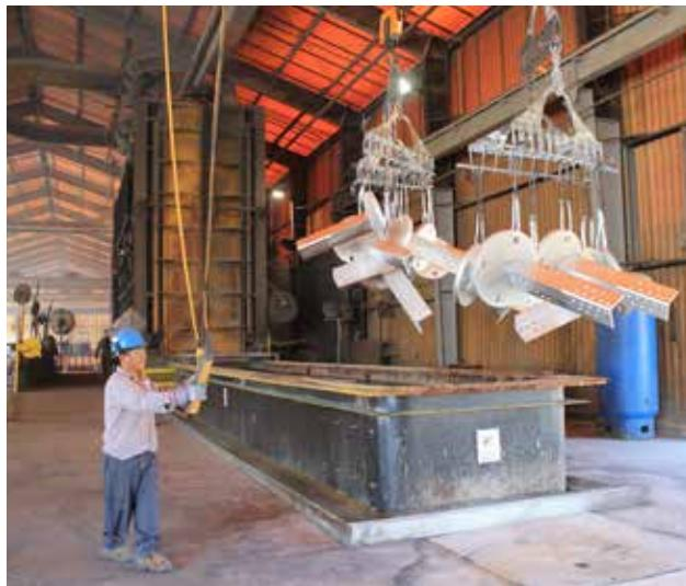
► Smaller elements, such as bolts, go through the galvanizing process in special spinner baskets in the 23-ft tank. After the zinc dip, the baskets are spun in a special machine to remove the excess zinc.
