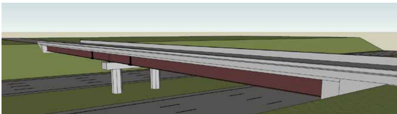
▲ Typical two-span overpass bridge.
