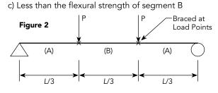
3 Given: From AISC *Manual* Table 3-6, the  $L_p$  value for a W18×35 beam is equal to 4.31 ft. The beam below has an unbraced length of 6 ft. True or False: The nominal flexural strength of the beam will be less than  $M_p = F_v Z_x$ .
