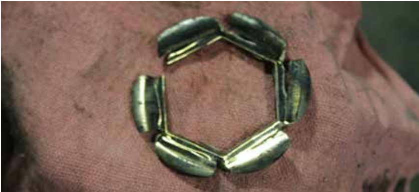
▲ A hexagonal punch-out, which becomes scrap.
