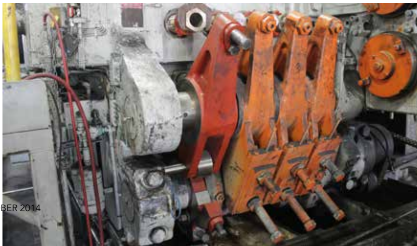
◀ A view of the kick-out tooling from the exterior of the machine.
