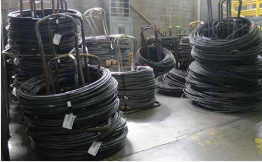
◀ Steel coil, in rolls, waiting to be turned into bolts.
