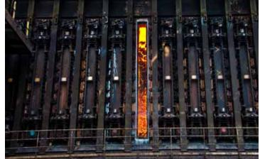
A batch of coke ready to be removed from a coke oven.
