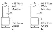
**3** True or False: When designing an HSS truss, one should try to use gapped K-connections instead of overlapped connections.
