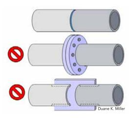
Tip 10 – When AESS requires a clean line, make it direct. ▼ Tips 14, 15 and 16 – When AESS is close to view, reduce the visual impact of the splices as much as possible.
