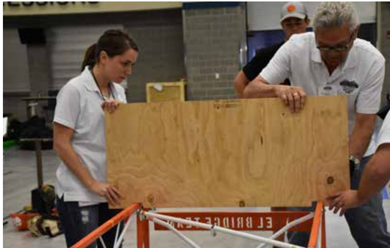
▼ The board test looks for elements projecting above the deck.
