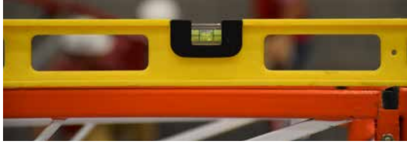
▲ Testing for levelness following the build portion.
