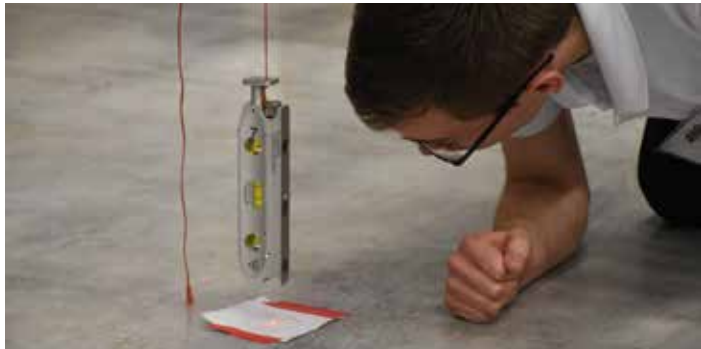
▼ Precisely measuring deflection following vertical loading.
