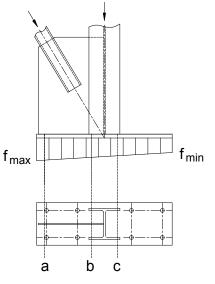
In practice, the presence of the gusset plate is typically neglected in the base plate design.
