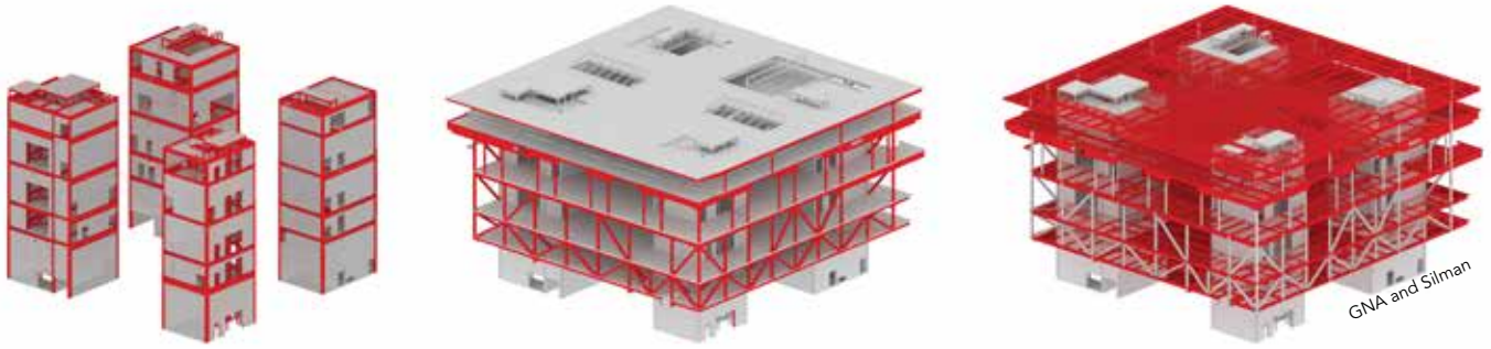
▲ Steel composite cores, perimeter trusses and floor framing.
