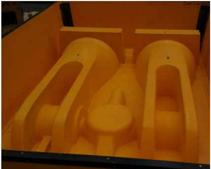
▲ Tooling for a universal pin connector casting.
