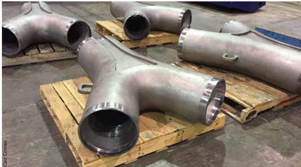
▲ A universal pin connector with an architectural taper.
