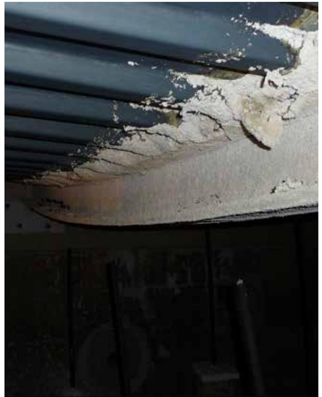
▲ An SFRM-protected floor assembly following a fire test.
