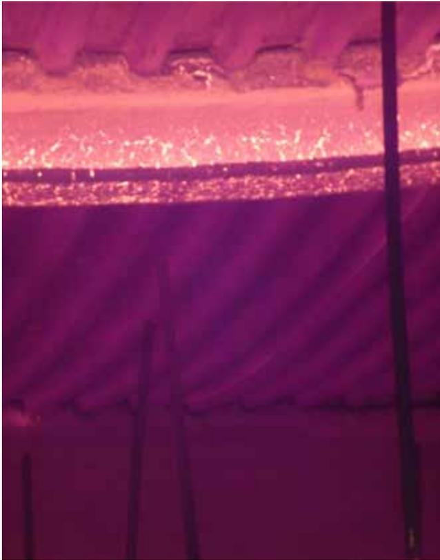
▲ A floor assembly undergoing a fire test.
