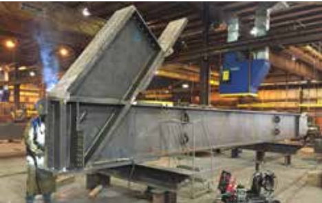
▲ A 60-ft-long diagonal section of a type 1 truss, a 65-ksi W36x925, being heat-straightened in the shop (which was done for most sections).
