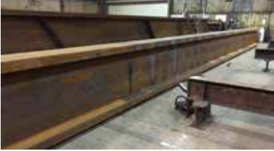
▲ A 60-ft-long diagonal section of a type 1 truss, a 65-ksi W36x925, being heat-straightened in the shop (which was done for most sections).
