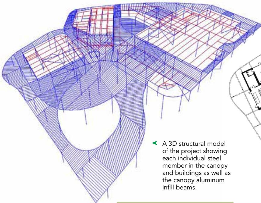
◀ A 3D structural model of the project showing each individual steel member in the canopy and buildings as well as the canopy aluminum infill beams.
