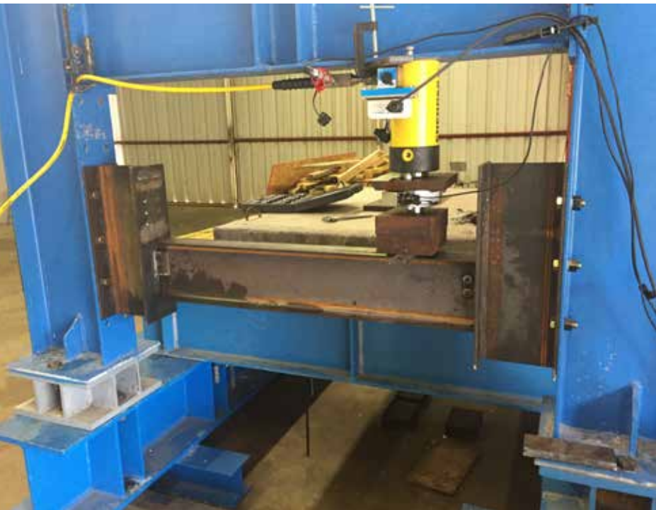
▲ Test setup for shear tab connection (left); failed beam in double-angle connection (right).
