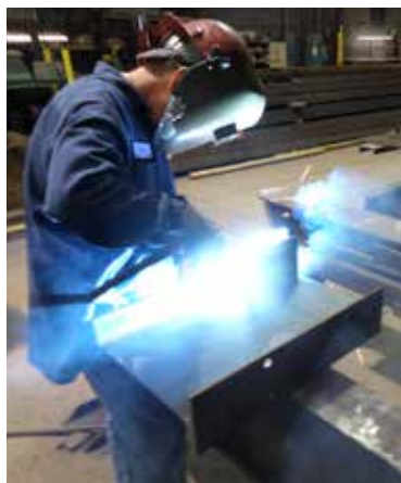
▼ Welding in a fabrication shop, using the FCAW-G process.
