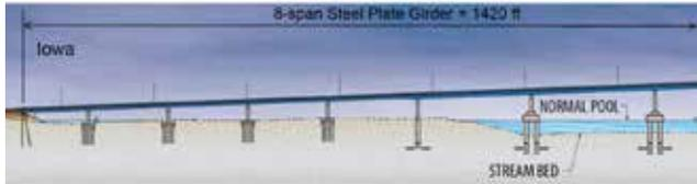
▲ The span layout of the new bridge.
