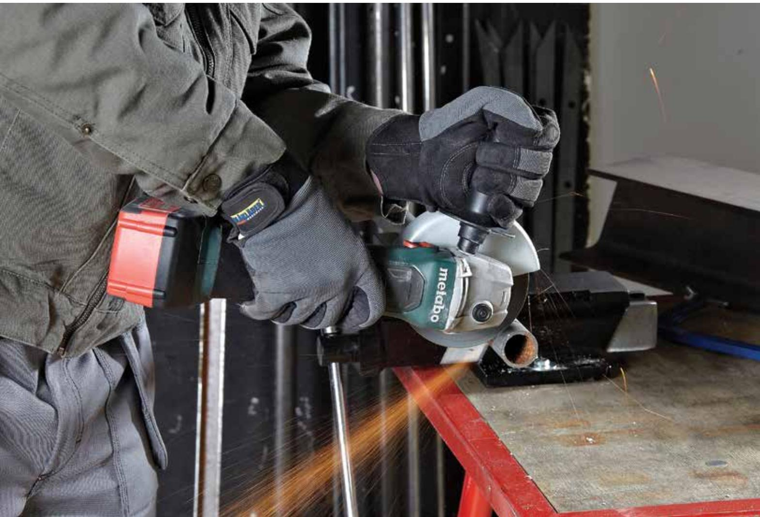
figure 3. When working with angle grinders, always secure your work with the proper vise or clamp, and don't overreach.
