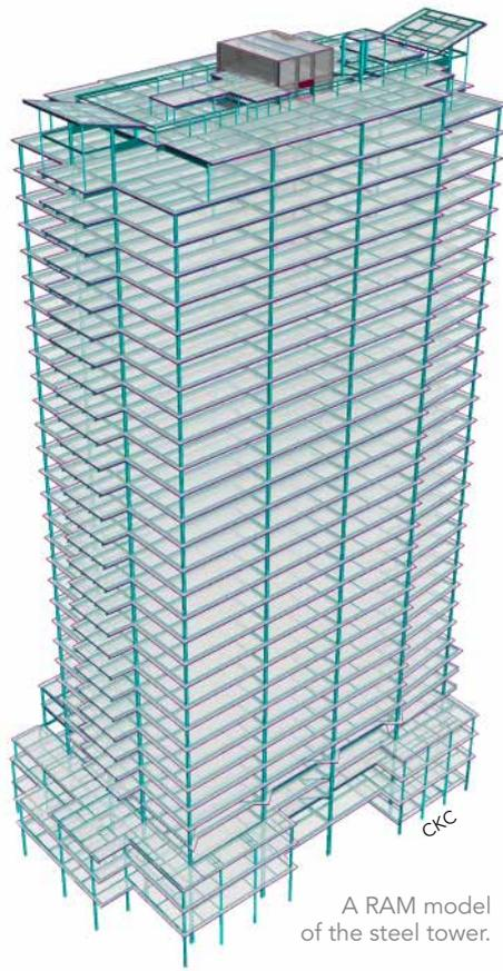
A RAM model of the steel tower.
