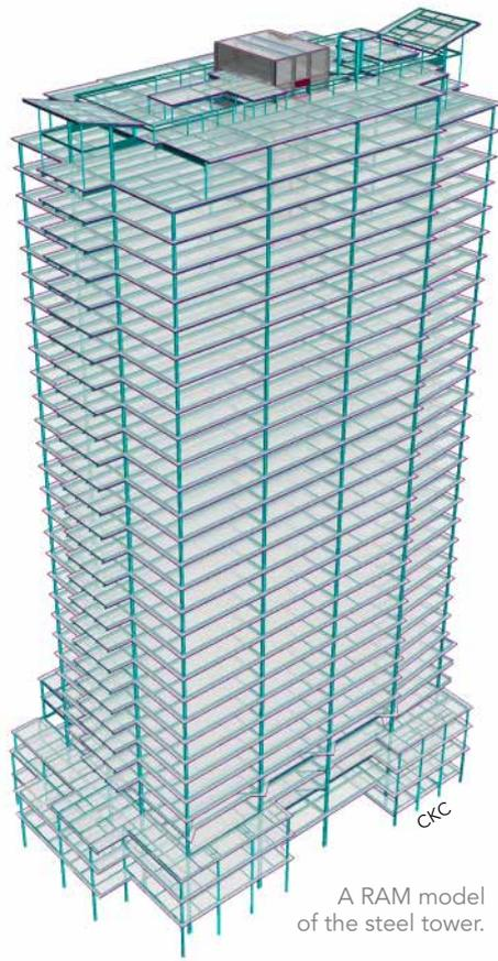
A RAM model of the steel tower.
