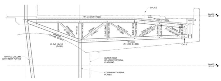
A sloping-column-to-truss connection.
