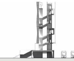
manufacturing. A series of customized unitized frames function as vertical supports running the length of the building, while a system of double-layered, stress-skinned floor plates comprises the horizontal structure. Lateral support is afforded by external skins and panels serving both structural and shading roles.
