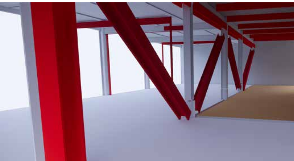
Multiple existing columns were removed at the first floor to create a new assembly space, and a story-deep truss was incorporated into a corridor wall on the floor above to transfer loads in the direction parallel to the long dimension of the new space.
