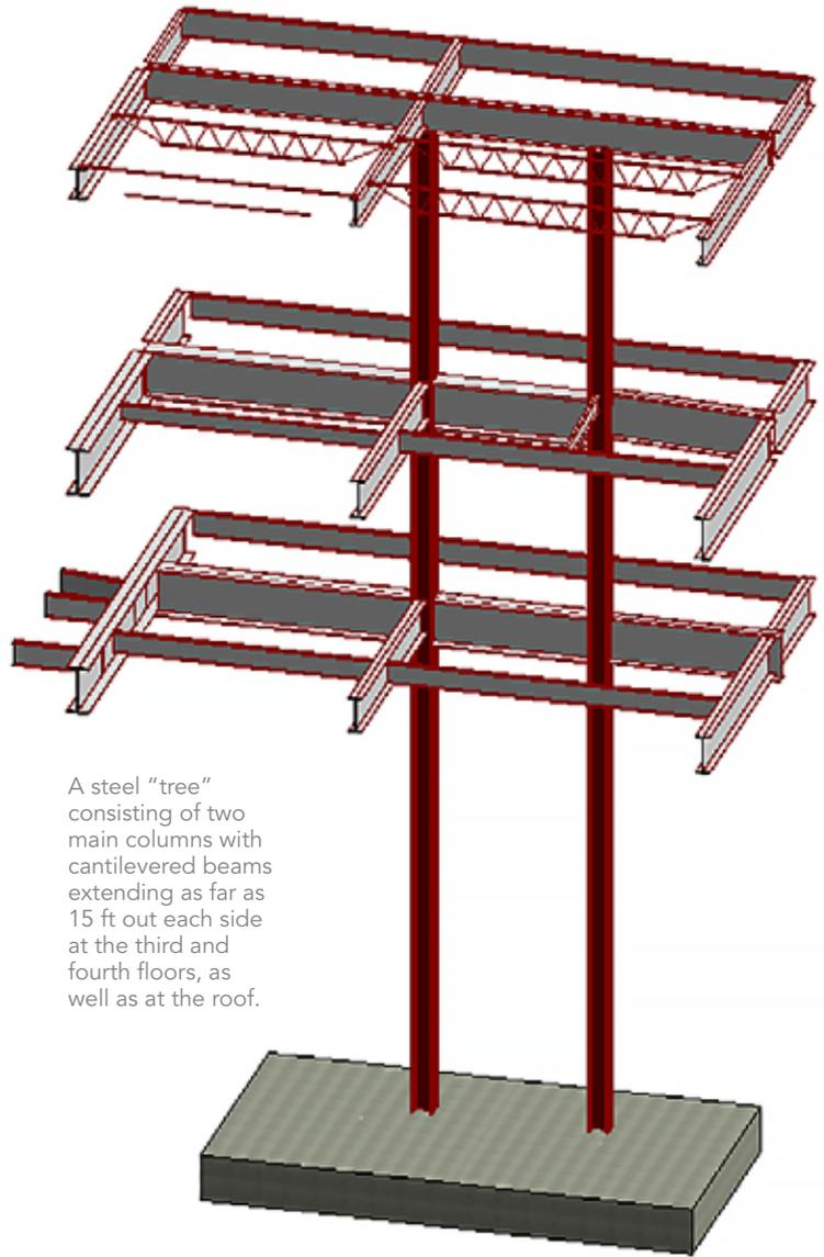
A steel "tree" consisting of two main columns with cantilevered beams extending as far as 15 ft out each side at the third and fourth floors, as well as at the roof.
