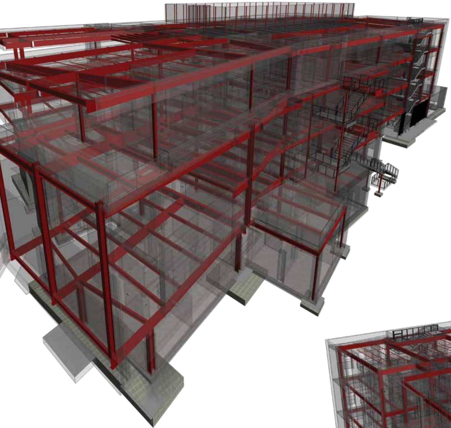
The structural system is comprised of composite roof and floor decks on a frame of ASTM A992 50-ksi steel beams and columns.
