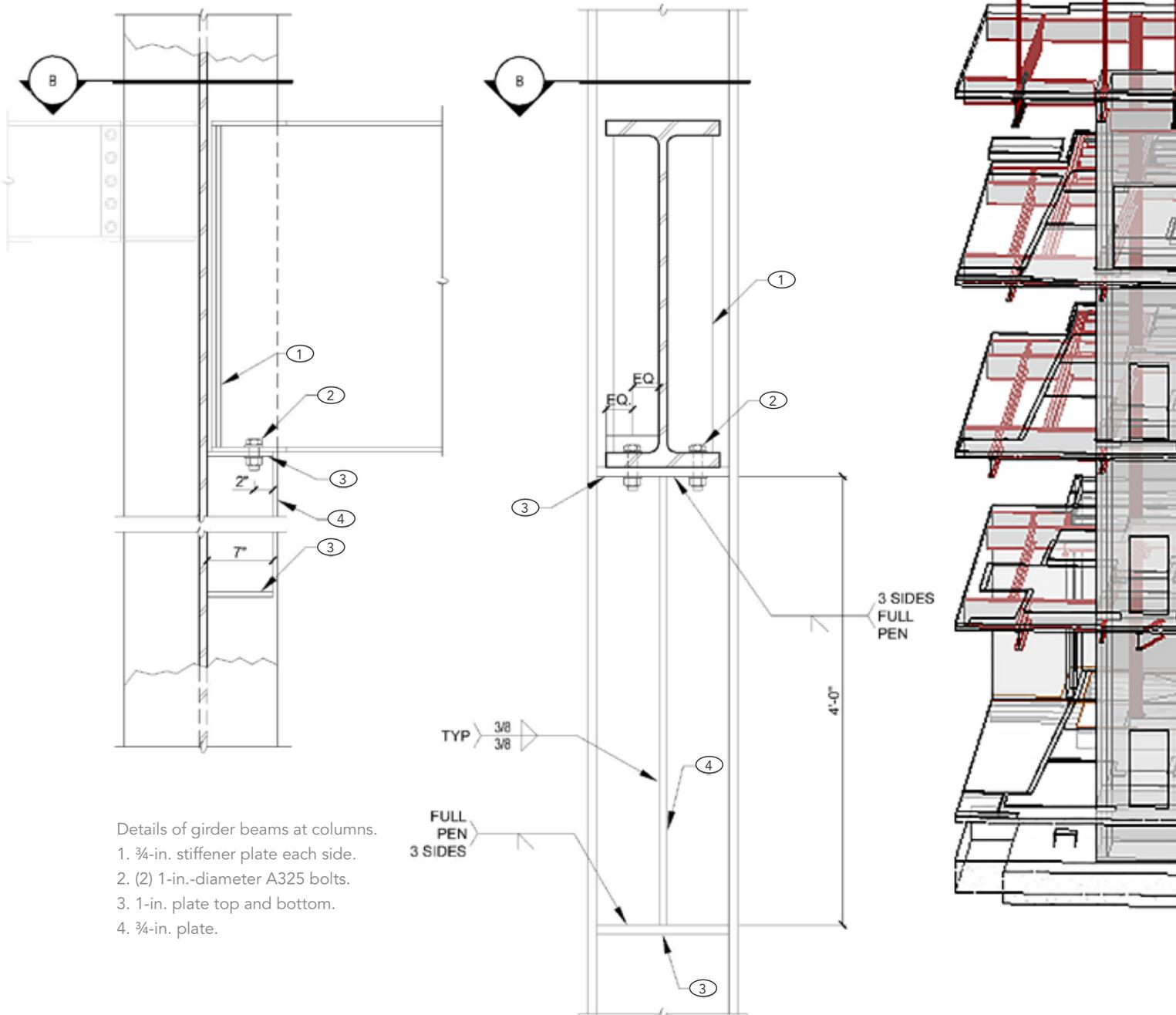
Details of girder beams at columns.
