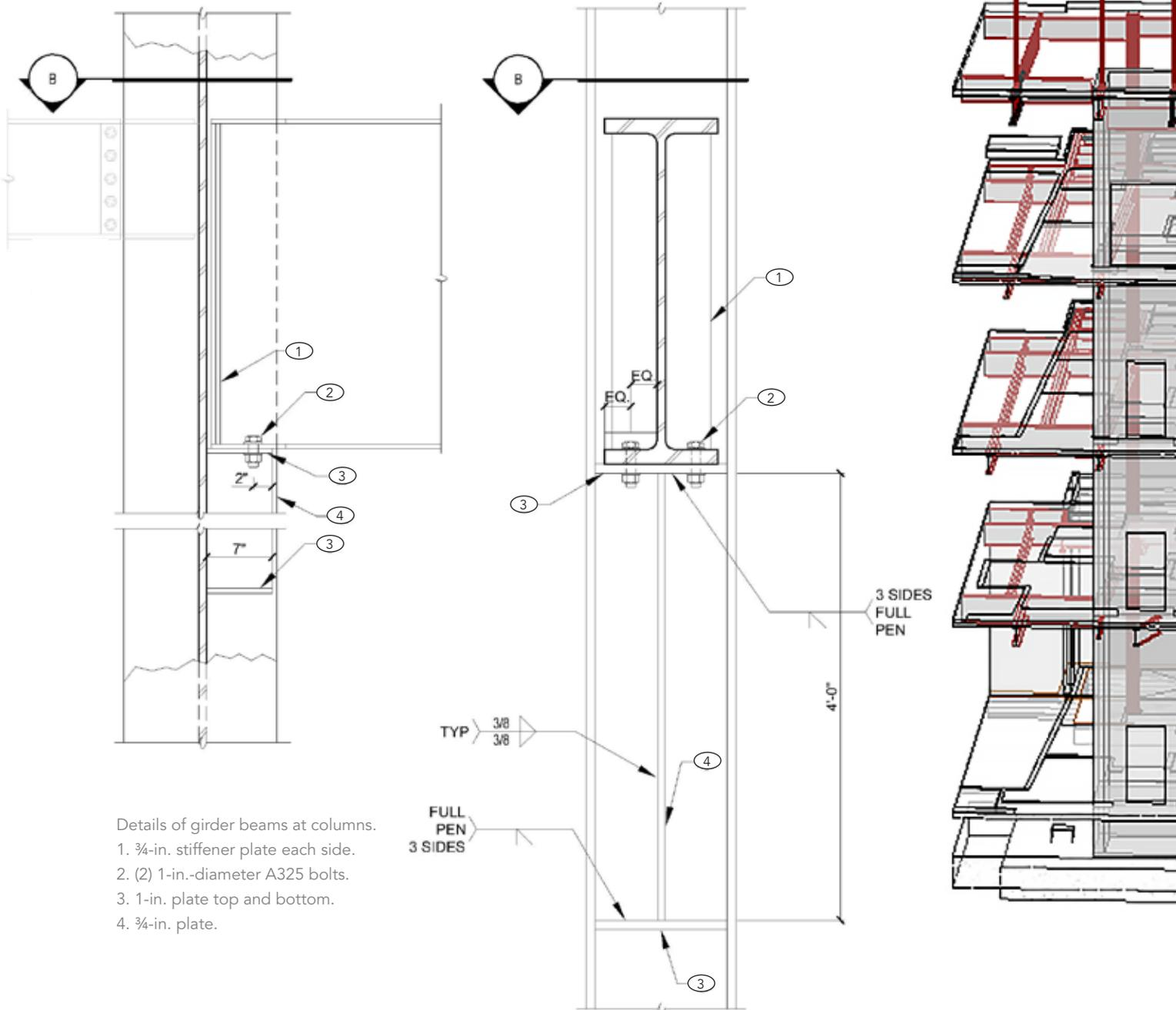
Details of girder beams at columns.
