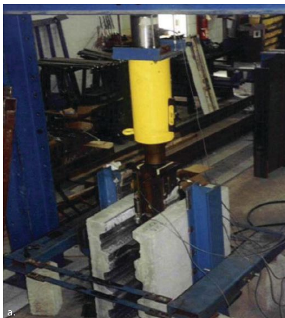
Figures 2a, a monotonic pushout test setup, and 2b, a new testing rig for cyclic and monotonic pushout tests.
