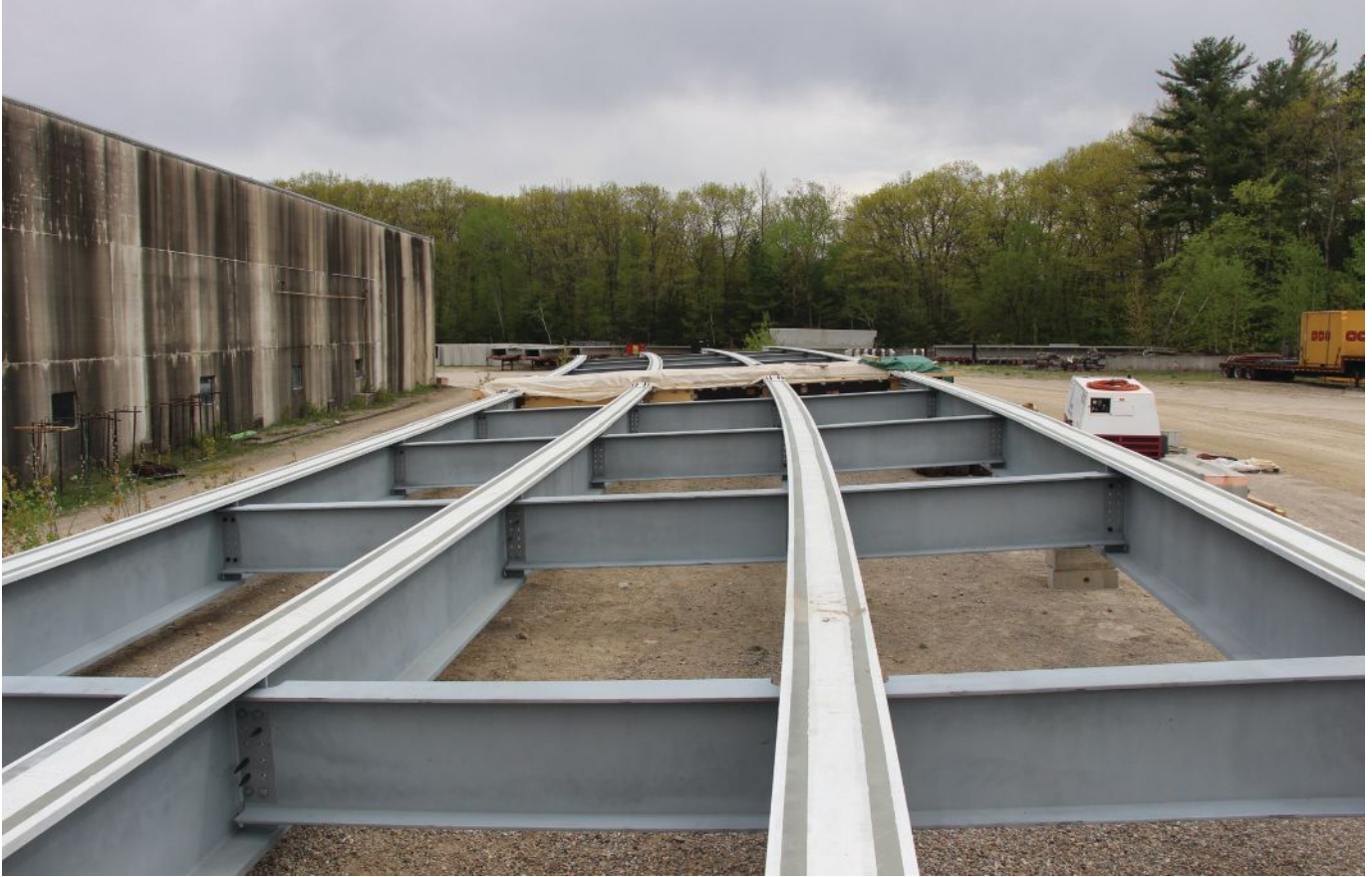
above: The full 103-ton steel superstructure.
