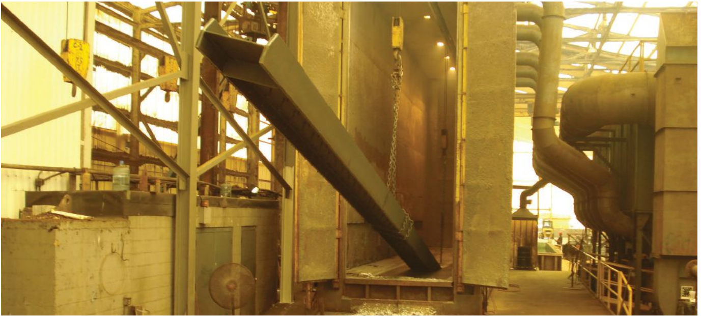
opposite page: Steel elements that are too large to be galvanized in a single dip can be progressive-dipped.
