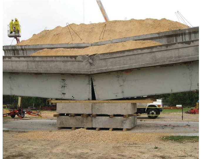
The study's third test, in which a bridge was incrementally loaded until it collapsed—after 182 tons of weight was placed on the deck.
