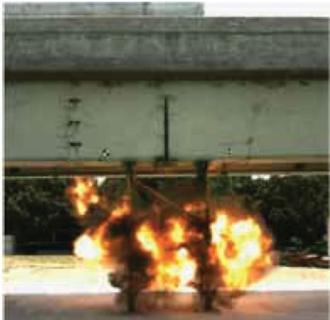
..... A test simulating a full-depth fracture of the outside girder webs of a twin-tub girder bridge.
