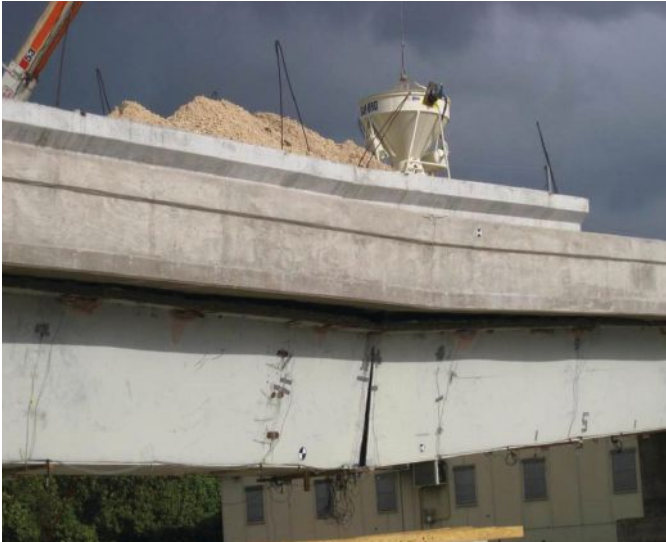
The study's third test, in which a bridge was incrementally loaded until it collapsed—after 182 tons of weight was placed on the deck.
