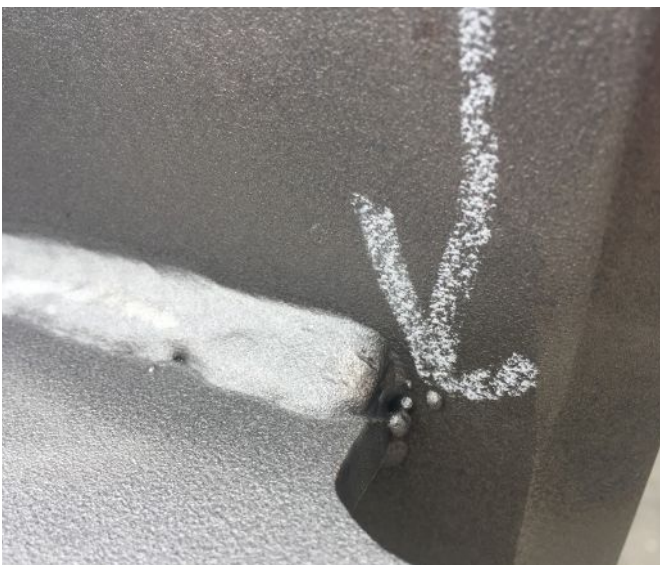
above/below: A site visit to a fabrication shop to inspect steel with AESS requirements. The weld spatter below will need to be addressed.
