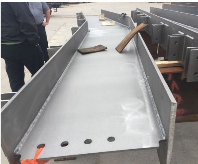
above/below: A site visit to a fabrication shop to inspect steel with AESS requirements. The weld spatter below will need to be addressed.
