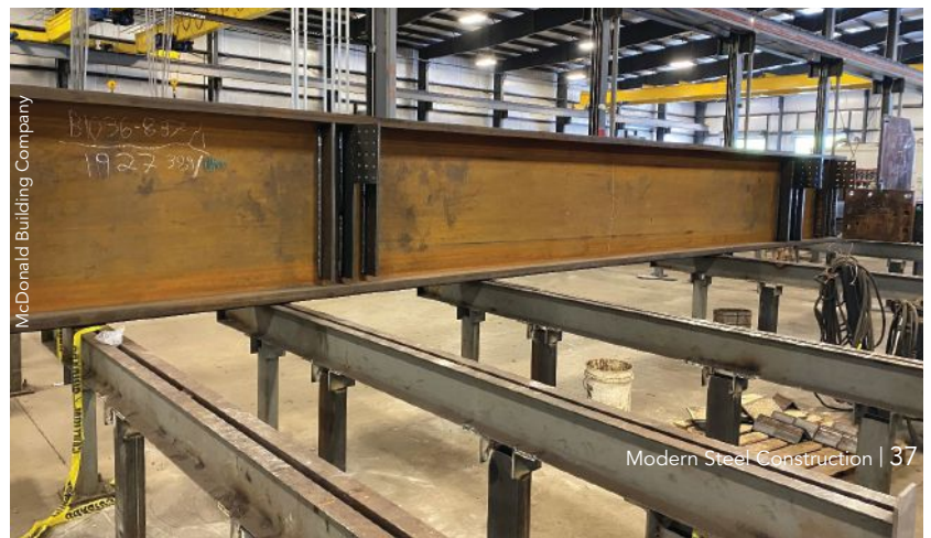
below: A completed transfer girder in the fabrication shop.
