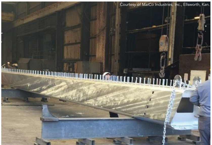
below: Hot-dip galvanizing is the preferred method of corrosion protection for FSPGs.
