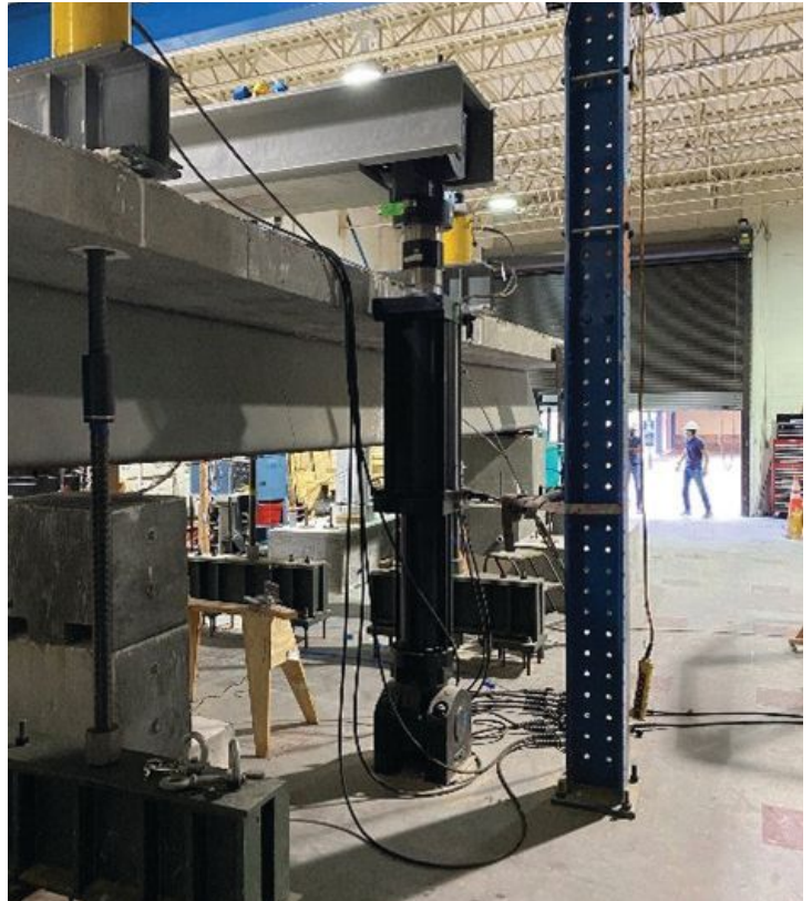
Fig. 3. Testing at FIU was performed to increase the maximum length of an FSPG bridge to 105 ft. The resulting load-deflection curve is shown below.
