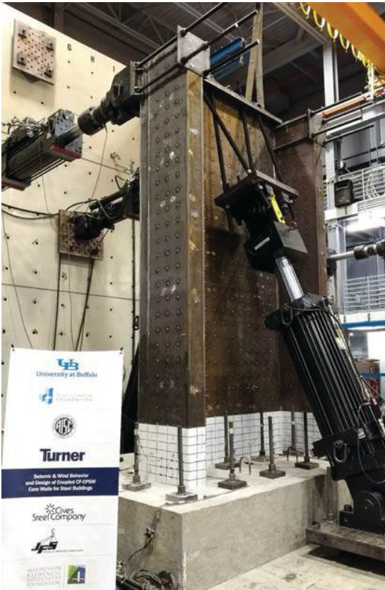
Fig. 5. University at Buffalo test Specimen for a C-shaped wall configuration.
