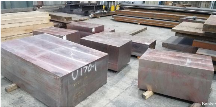
above and below: Forged steel nodes in the Tekla model and at Banker's fabrication facility.
