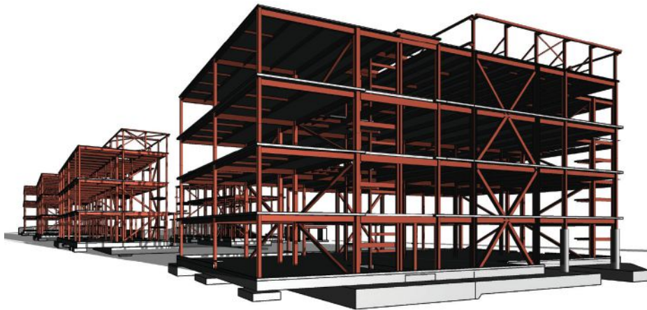
below: A 3D model of the framing system. The most common beam size used is W16x26.
