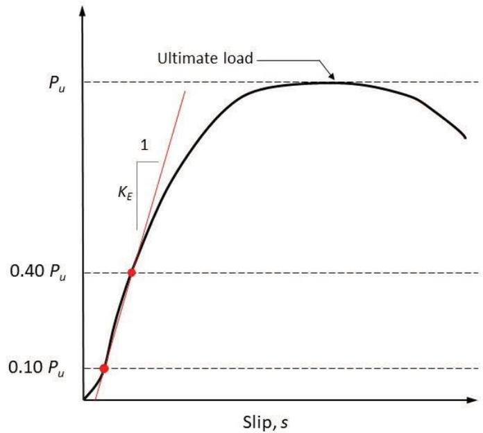
Fig. 4. Shear connection elastic stiffness,  $K_E$ .
