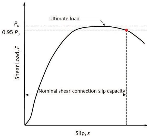
Fig. 3. Shear connection ductility.
