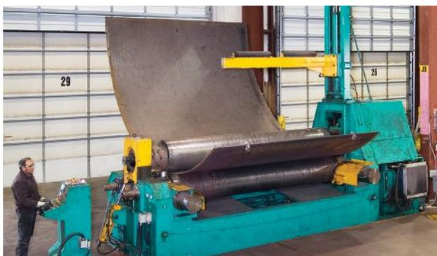
2" x 12' plate roll can roll 40' lengths
