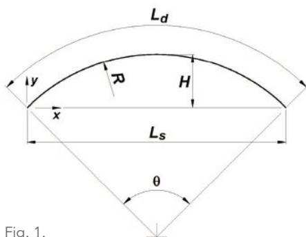
Fig. 1. Circular geometry.
