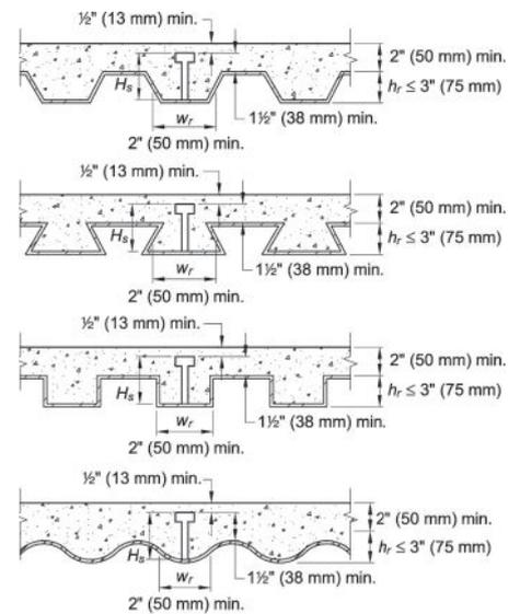
Fig. 2. Steel deck geometries and limits.
