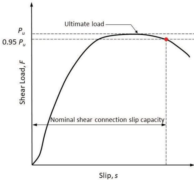
Fig. 3. Shear connection ductility.
