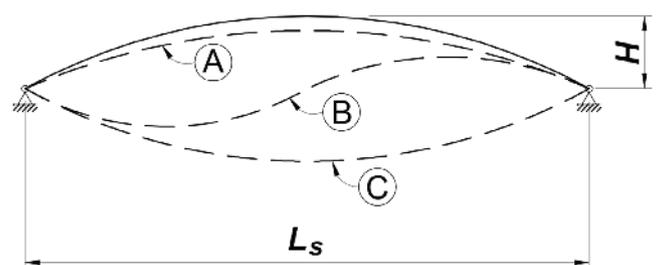
Fig. 2. Shape A shows the deflected shape at imminent buckling. Shapes B and C show snap-through buckling that can occur in a symmetric mode or asymmetric mode.
