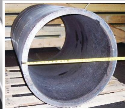
1 1/2" plate 45" long rolled to a 25" inside diameter
