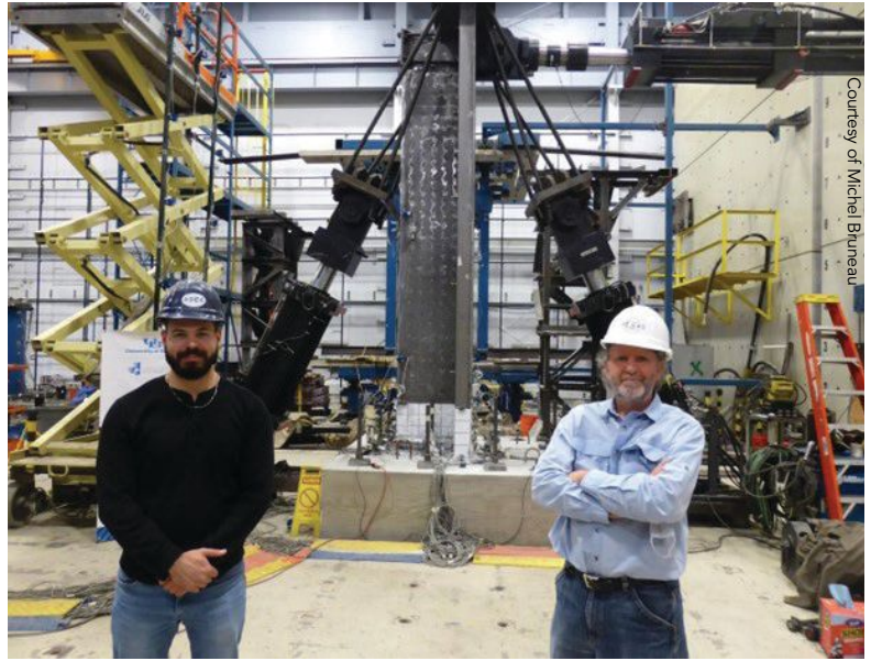
above: Former PhD student (and current structural engineer with Thornton Tomasetti) Emre Kizilarslan and SUNY Distinguished Professor Michel Bruneau proudly displaying their T-shaped SpeedCore test specimen at the University at Buffalo.
