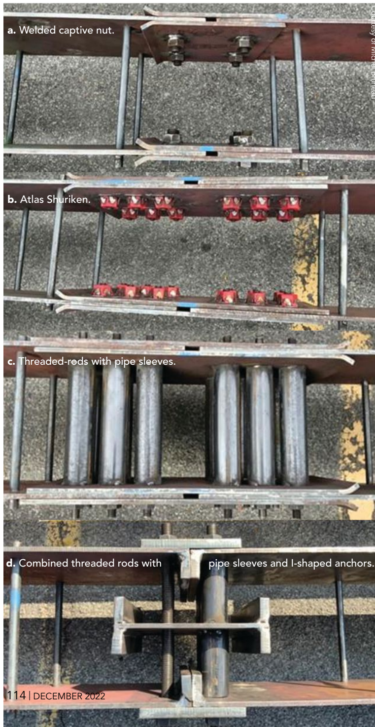
below: Various bolted splice tension specimens prior to placement in their test fixtures on a SpeedCore sample.
