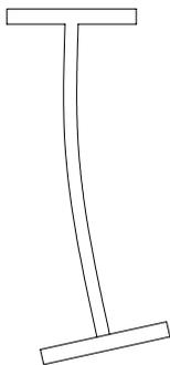
Section J10.4: Web Sidesway Buckling states: “When the required strength of the web exceeds the available strength, local lateral bracing shall be provided
