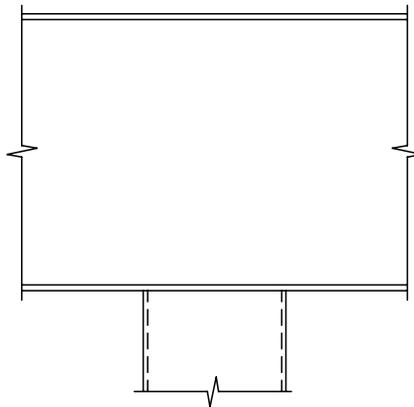
Section J10.7: Unframed Ends of Beams and Girders states: “At unframed ends of beams and girders not otherwise restrained against rotation about their
