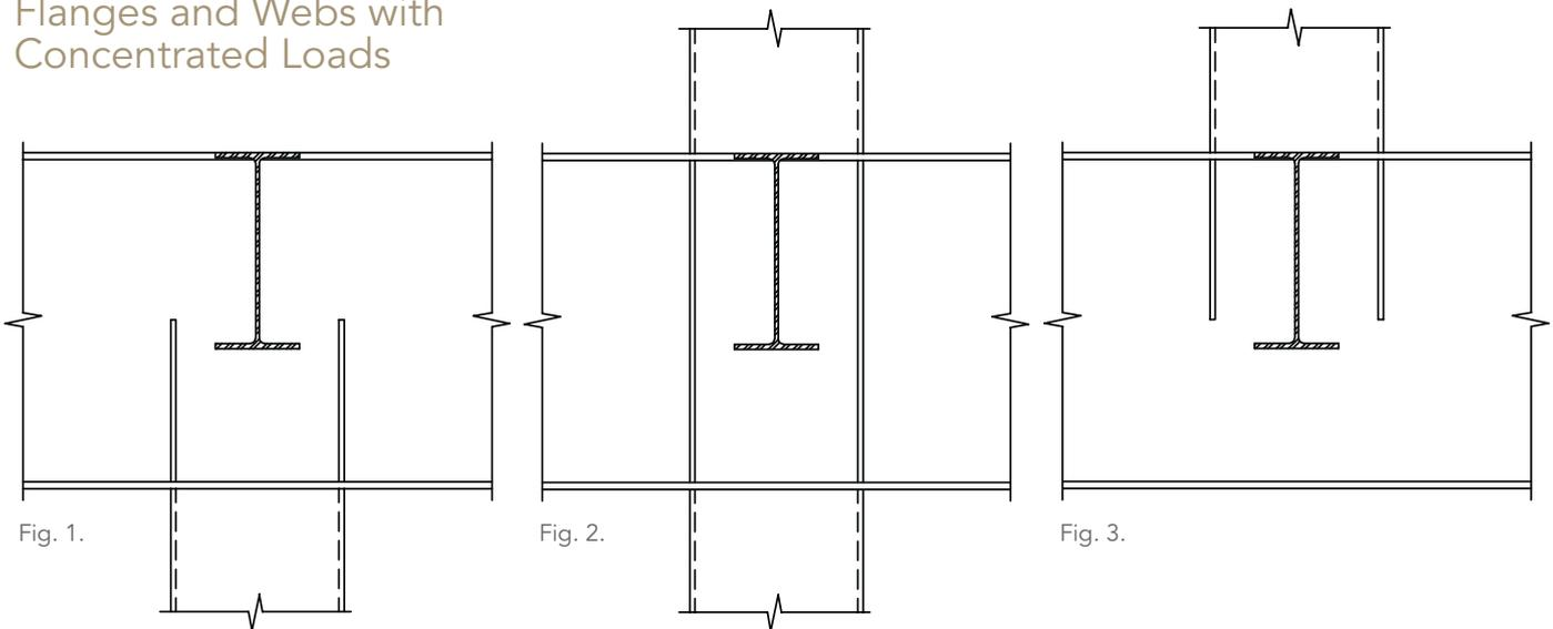
**Looking at Figure 1, should web compression buckling be checked per the requirements of Section J10.5 of the AISC Specification for Structural Steel Buildings (ANSI/AISC 360)?**
