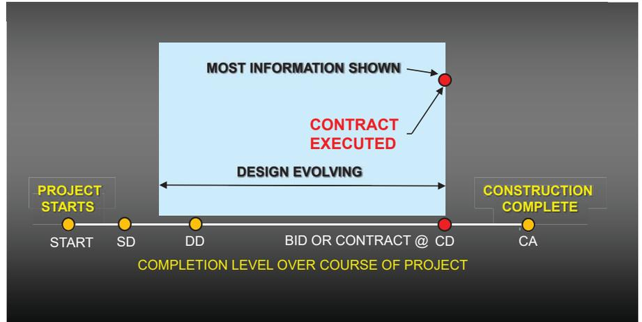
Fig. 1. The typical construction sequence before the fast-track approach became more common.
