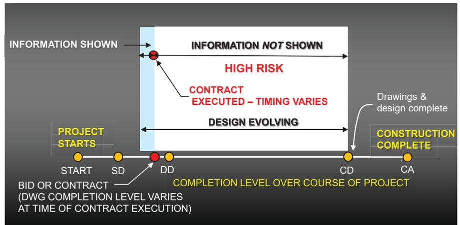
Fig. 2. The modern fast-track construction process.
