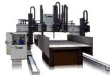
CNC Gantry Drilling Lines
