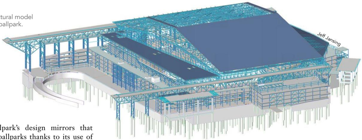
The ballpark's design mirrors that of historic ballparks thanks to its use of exposed structural steel. With this traditional approach working in concert with modern-day elements like the ETFE retractable roof, Globe Life Field has stepped up to the plate as the lead-off hitter for a new era of ballparks. ■
