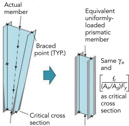
Fig. 1. Equivalent uniformly loaded prismatic member concept.
