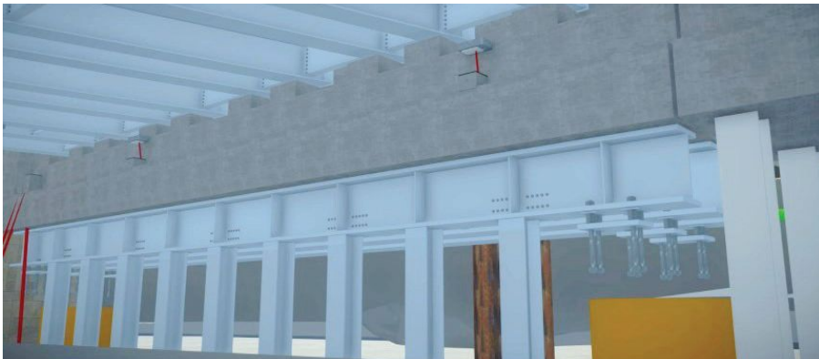
above: A 3D model showing the steel beam system located beneath the abutments of the East 138th Street Bridge.
