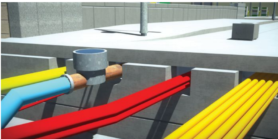
below: A 3D model showing utilities underneath the bridge.
