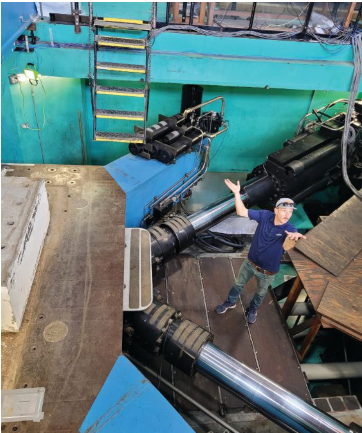
below: The seismic response modification device (SRMD) facility showing the shake table platen and large hydraulic actuators.
