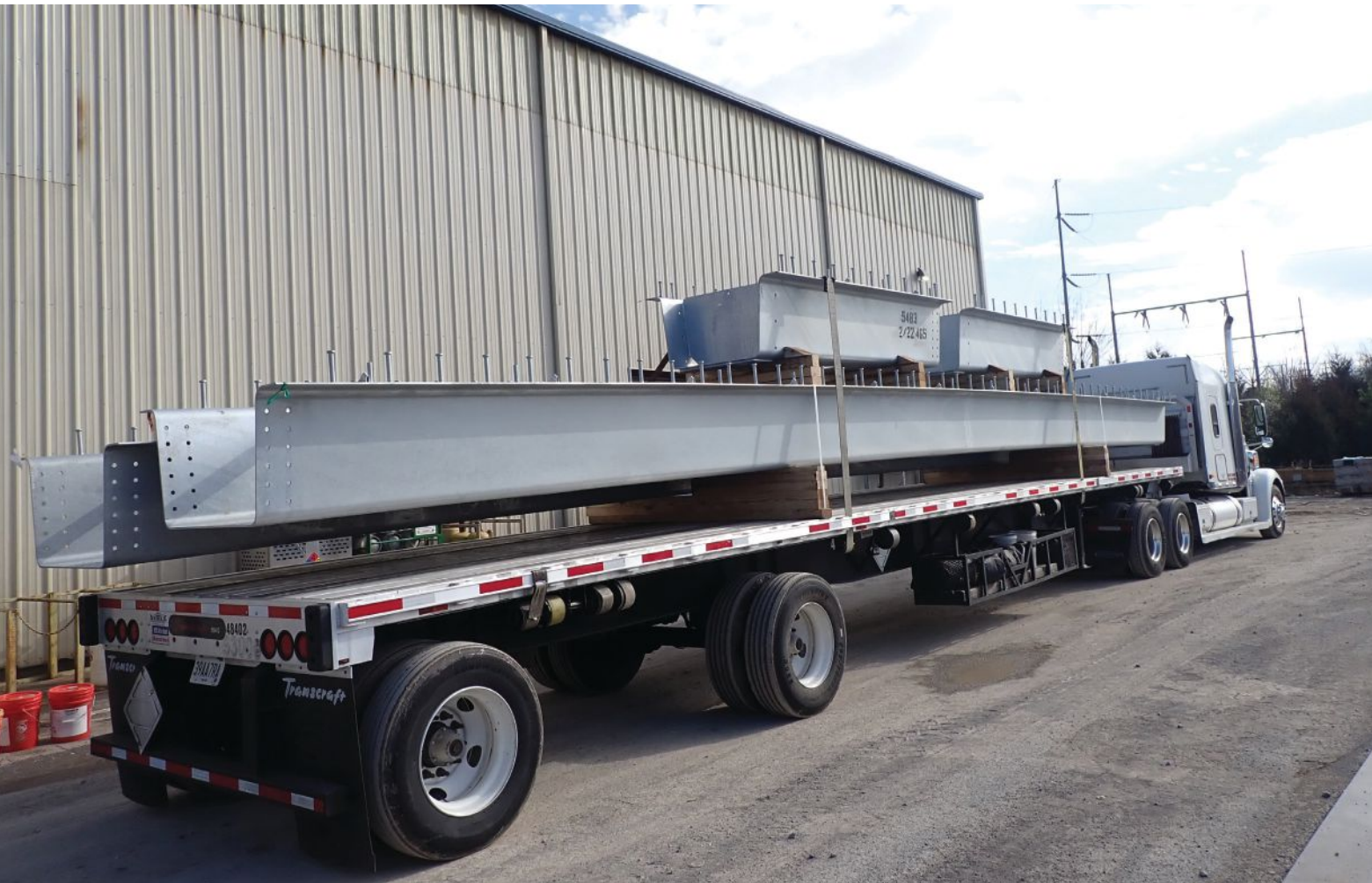
below: Tub girders being transported to one of the Michigan projects
