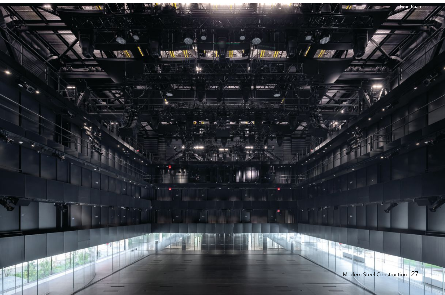
above: The side gantries can move 10\frac{1}{2} ft toward the center of the hall, and the rear gantries can move up to 44\frac{1}{2} ft toward the stage.
