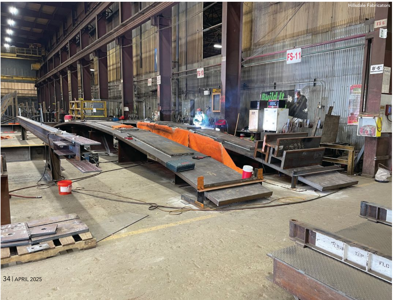
above: A half-arch segment before shipment to the jobsite.
