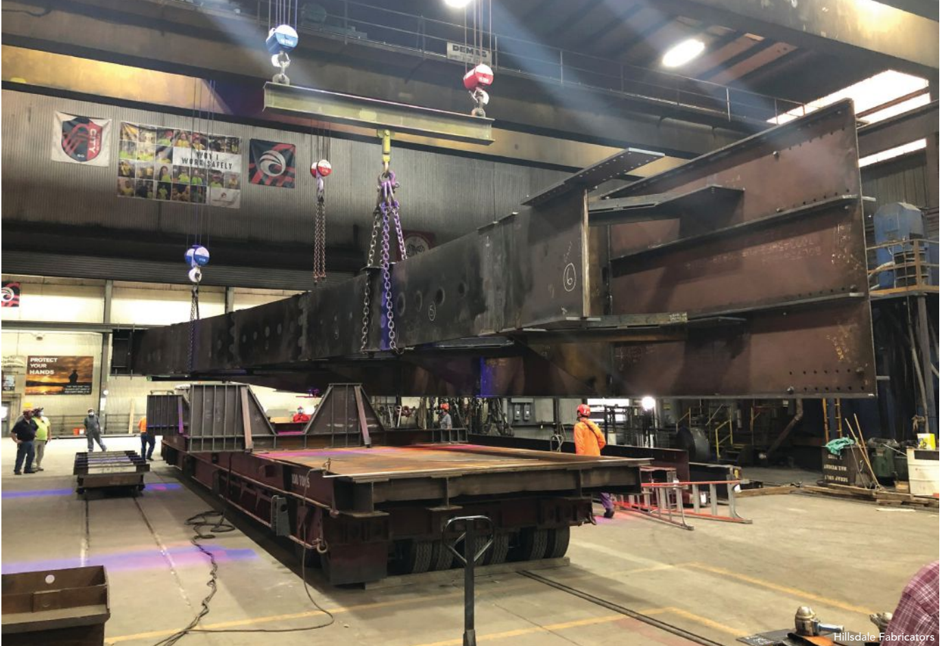
above: A half-arch segment before shipment to the jobsite.
