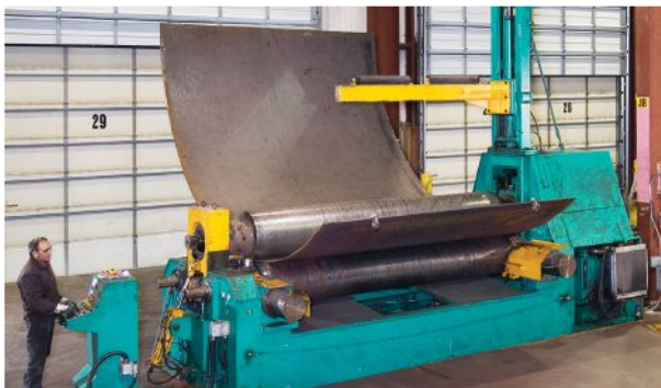
2" x 12' plate roll can roll 40' lengths
