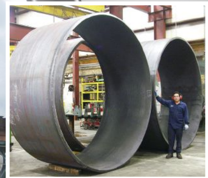
2" x 58½" beveled plate rolled to a 128" outside diameter
