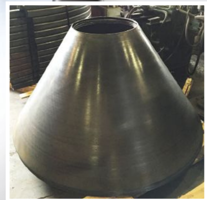
5/16" plate cone with a 16" minor diameter and a 48" major diameter with an overall height of 42"
