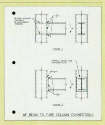
(flange forces), thickness and width of the column wall, and width of beam flange in comparison to the width of the connecting face of the tube.
