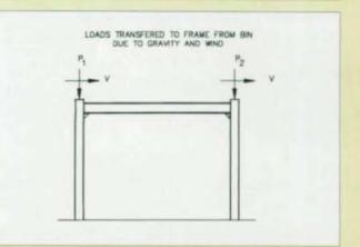
rigid frame action. The maximum moment that occurs at the connection is caused by both the lateral shear and shear due to the sidesway associated with unsymmetrical gravity loading.
