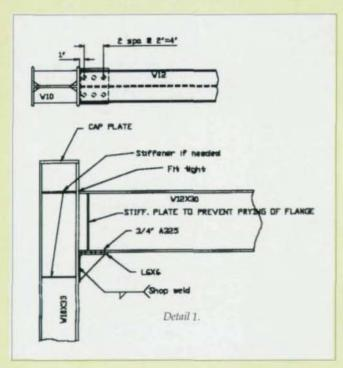
of the angle, and tension in the bolts. The moment is then transmitted to the column by shear stress in the shop weld.
