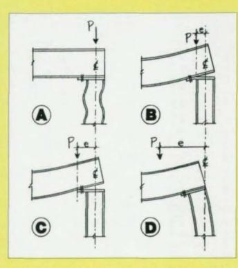
provide a system complex enough for illustrative purposes. In the hypothetical detail shown, the eccentricity is a function of the designed relative stiffness of the various components.
