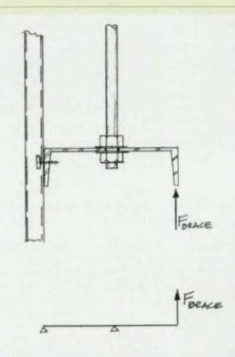
channels. These members are usually continuous over the column supports, since lap splicing can be easily made, and the points of inflection are frequently assumed to be braced laterally.
