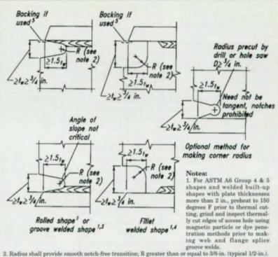
Access opening made after welding web to flange
