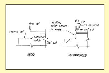
The AISC Manual of Steel Construction Load and Resistance Factor Design, Volume II (1994) recommends on page 8-225 that an approximate minimum radius to which the re-entrant corner of a beam cope must be shaped is <sup>1</sup>/<sub>2</sub> in. While there is nothing magical about a 1<sup>1</sup>/<sub>2</sub>-in. radius, this value is recommended to emphasize that square-cut corners and significantly smaller radii do not provide the smooth transition required.
