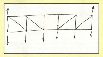
Theoretically, all joints for trusses are assumed to be pinned connections, so this truss without a diagonal member in the center panel is virtually a mechanism instead of a structure. Besides, there is no force (there is no need for the diagonal member in this case) on the diagonal member only if the loading condition is perfectly symmetrical. This situation is too ideal in practice, so there is need for the diagonal member to make a stable truss design.
