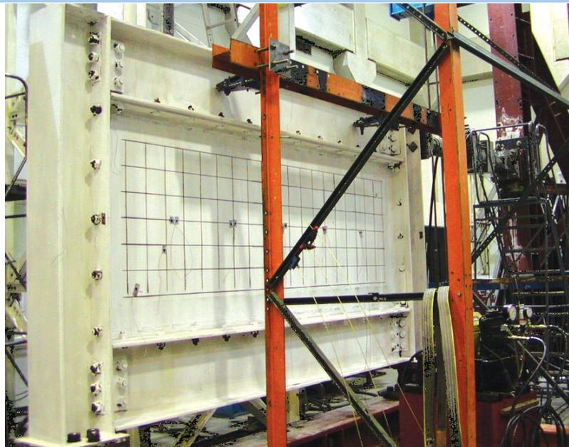
Steel plate shear walls have been tested extensively. A shear wall specimen, above, is readied for testing. After testing, below, the diagonal fold lines of the buckled web are readily apparent.
