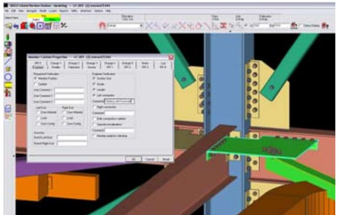
**Figure 4:** Various electronic forms allow reviewers to attach comments and approvals as part of the electronic model, although the model itself cannot be changed by the reviewer.
