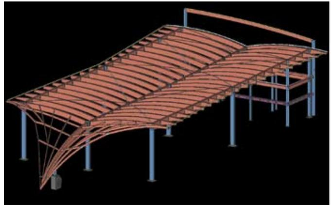
**Figure 2:** Individual elements of this information-rich 3D model of curved framing are shown as they relate to the rest of the structure, rather than as individual, isolated 2D drawings.
