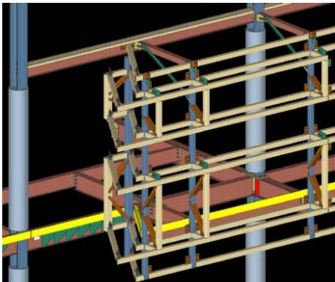
**Figure 1:** The availability of a 3D model can help reviewers visualize complex 3D relationships among structural steel members that otherwise might have to be inferred.
